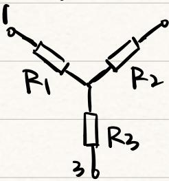
$$R_{12} = \frac{1}{R_3} (R_1 R_2 + R_2 R_3 + R_3 R_1)$$
